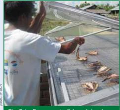
The Solar Dryer can dry fish or shrimp in as little as six or seven hours.
