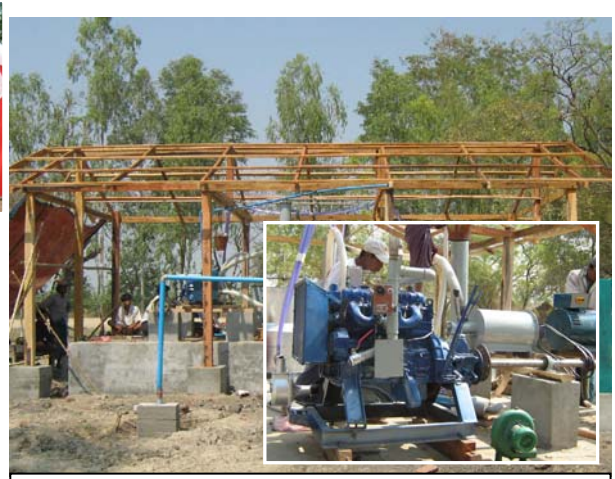
A Paddy Husk Bio-gas Power Generation (Mon Taw Gyi Village): Bio-gas from charcoaled husk can run diesel engine, thereby generating electricity for the 380 households there.
